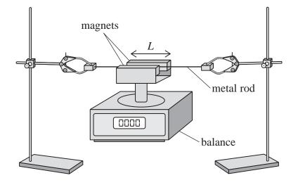
When the switch was closed, the reading on the balance increased by 2.8 g. The reading on the ammeter was 3.6A.
