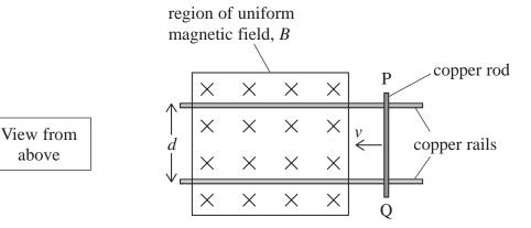
The rod and rails are in a uniform magnetic field that is directed vertically downwards.
