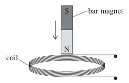
The coil was attached to a data logger. The data logger recorded the variation of e.m.f. across the coil with time.
