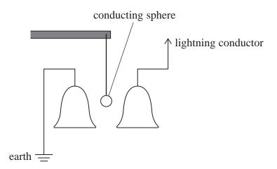
The lightning conductor is a long wire, attached to the top of a building. The lightning conductor becomes positively charged when in an electric field.
