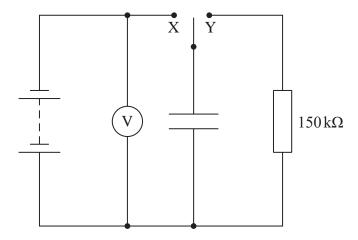
The student connected the switch to X to charge the capacitor. She then connected the switch to Y so that the capacitor discharged through the  $150\,k\Omega$  resistor.
