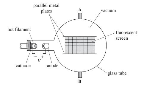
The beam is aimed at a fluorescent screen inside the tube and the path of the electrons is seen on the screen.
