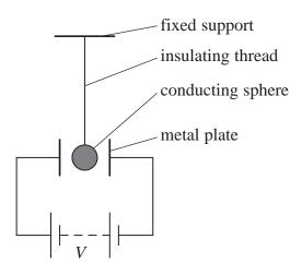
(a) There is an electrostatic force on the sphere when the sphere is charged.
